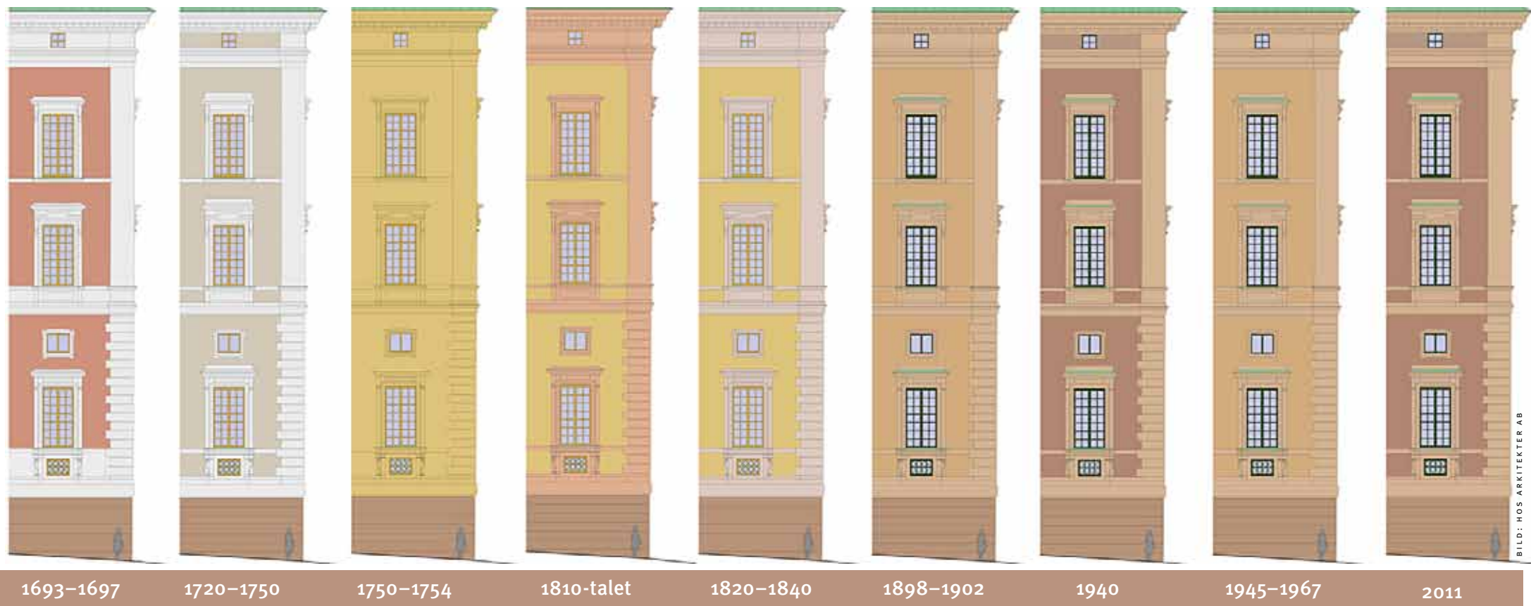
The colour of the Palace through the ages. The dark colours in 1940 and 2011 are not the result of re-painting, but of dirt.
